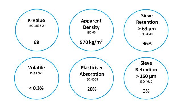
Note: The property data shown above has been obtained from laboratory tests on representative samples of VYNOVA<sup>TM</sup> S6806 polymer. Although the values are typical, they are for guidance only, and must not be used as a basis for specifications.
